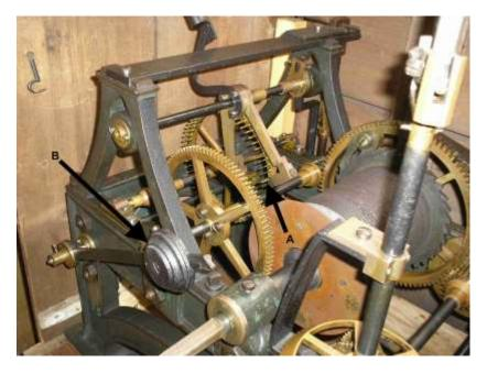
The striking train is on the right of the clock mechanism and on the quarters strikes one, two or three 'ting-tangs' on the two bells in the cupola on the top of the clock tower. On the hour the number of hours is struck on the larger bell.
